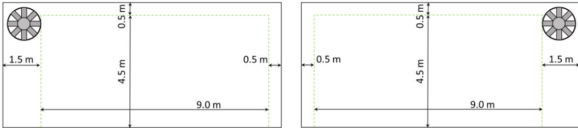
**Figure 8:** Cross sections of the tunnel.
