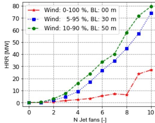
**Figure 16:** Critical HRR for different back-layering lengths and wind pressures.
