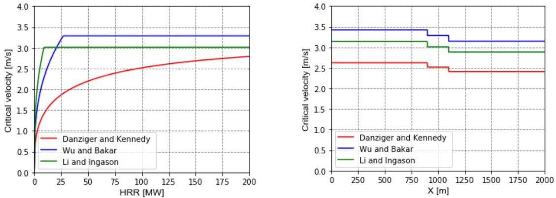
**Figure 1:** Critical velocity as function of the HRR and of the fire location.
