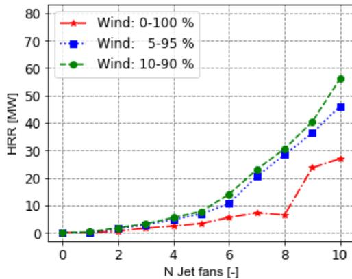
**Figure 15:** Critical HRR for different wind pressures.
