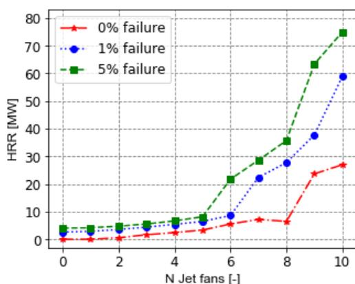
**Figure 13:** Critical HRR for different failure probabilities.
